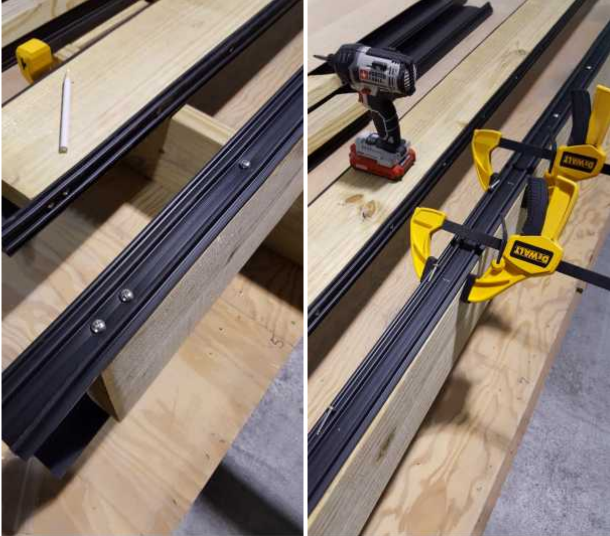
FIG 3 Left, Note the screw placement for the end of the bunk board. Right, Attaching the cover with screws along the side
