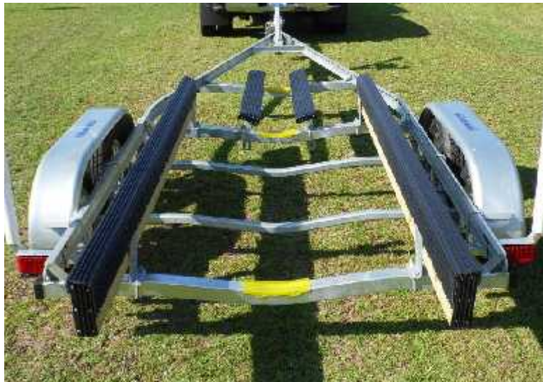
FIG 3.2 Additional screws installed to secure excess cover width. If desired cover can be trimmed to any final width. Ensure all screws are mounted within the channels and away from any facing that contacts the hull. Stainless Steel Staples can be used as well (not shown) as the primary mounting is done with the recommended screws.
