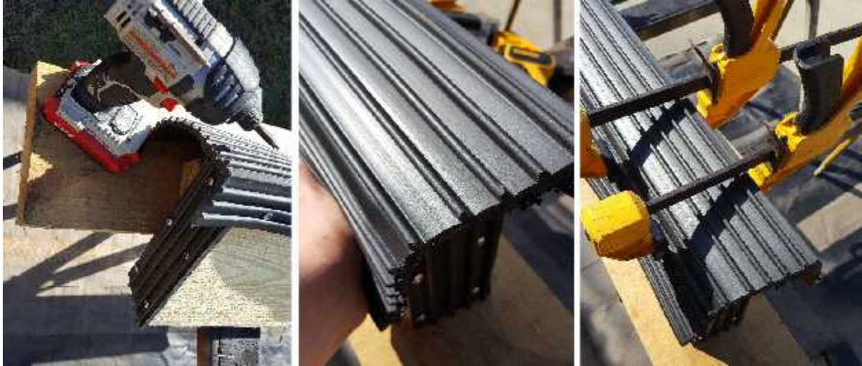
FIG 3.0 Left, Note the screw placement for the end of the bunk board. Right(2), Attaching the cover to the front of beam, Screws should be placed on last row or two of ridges along front side, far and away from any possible contact point with hull.
