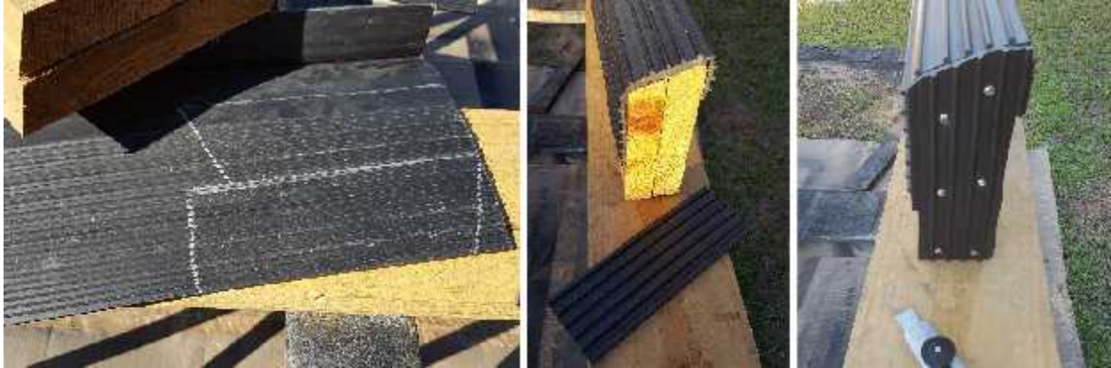
FIG 4 Use the end of the bunk Beam to create the pattern that you need for your end cap, once mounted trim the End of the cover or cap to complete the fit.
